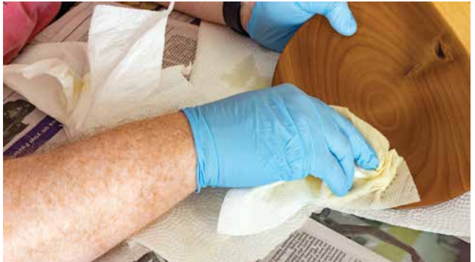
Wiping off excess finish
