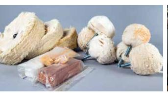
There are many sizes, shapes and grades of buffing wheel available alongside myriad forms of abrasive and finishing compounds to apply to the wheels. For manipulating or applying finishes, loose-fold wheels are most commonly used
