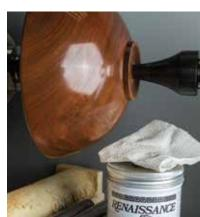
Wiping on a thin layer of microcrystalline wax and then the result once buffed off
