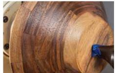
Using 0000 steel wool dry with soft circular motions takes little effort take any high gloss back as desired to any desired level down to matt
