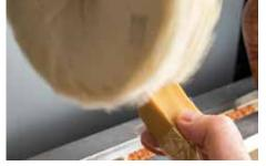
Once the wheels are prepared, load with either a wax finish or an abrasive compound. Each wheel should have a designated use for a certain task, you should not mix finishes and abrasives on any given wheel. It might be prudent to label what each buffing wheel is loaded with and used for
