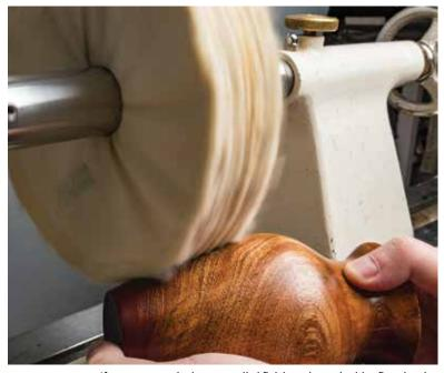
If you want, manipulate an applied finish on the work with a fine abrasive compound and, if desired, follow this by using a wheel or buffing pad loaded with a wax compound or finish to achieve a glossy effect
