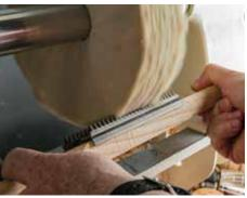
It is best to dress, also known as conditioning, the wheels with a wire brush or special toothed comb prior to loading or charging the wheel with a finish or abrasive compound. Charging the wheel is best done lightly and as needed. Always err on applying too little rather than too much abrasive or finishing compound on a wheel
