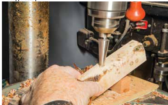
Fixturing for safely done angled drillings can be quickly done with scraps and hot-melt glue
