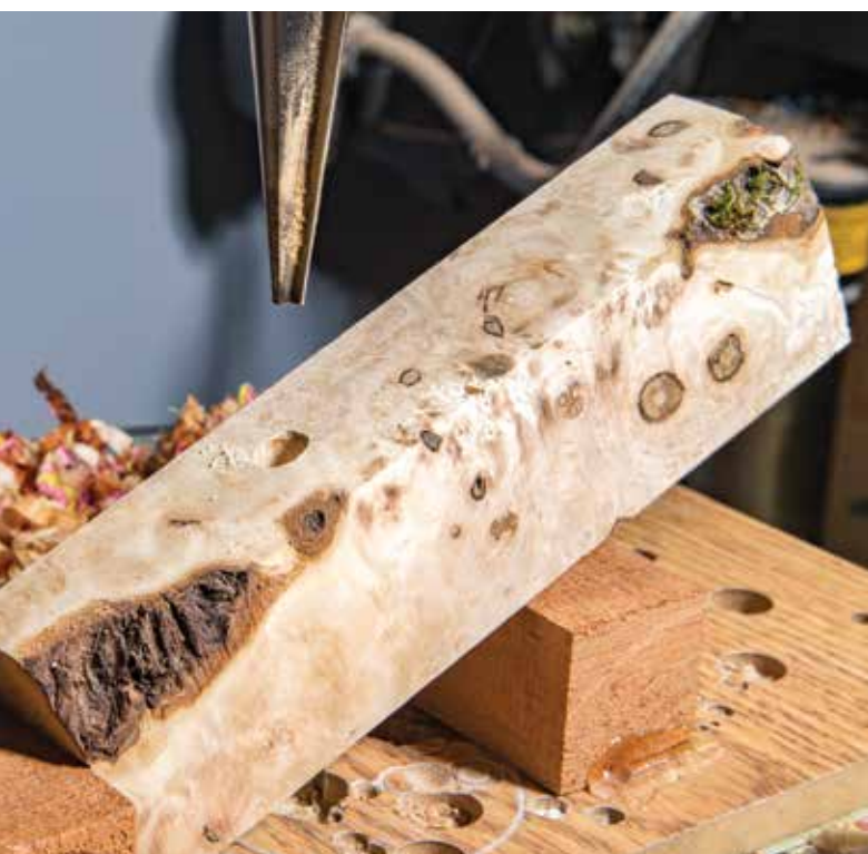
A starter drill for location followed by a body drill will set things well for the tapered reamer
