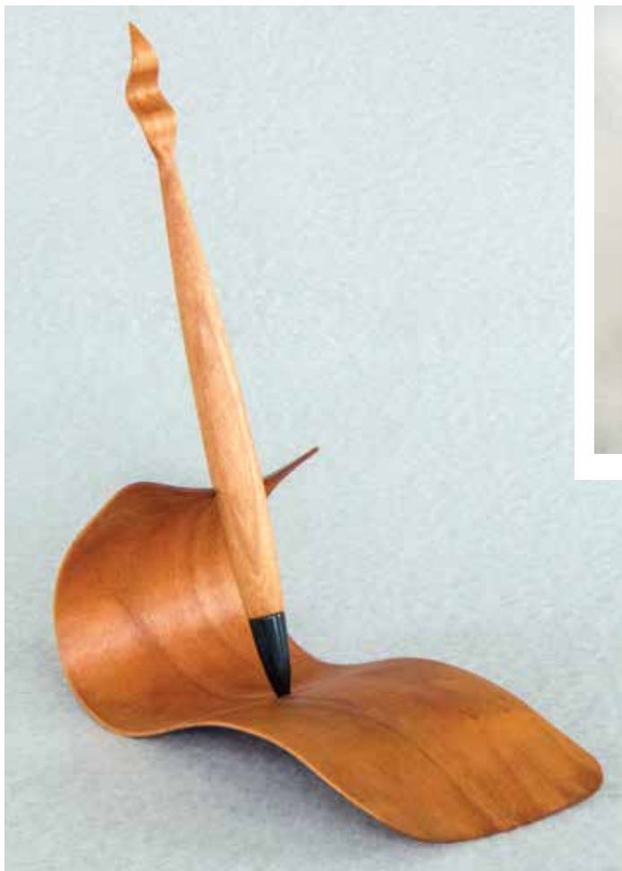
A different look at the pair. Yes, the curves in the pen were steam bent. Far more challenging than the stand
