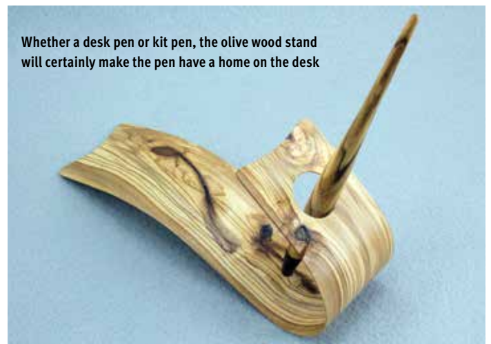
A different look at the pair. Yes, the curves in the pen were steam bent. Far more challenging than the stand
