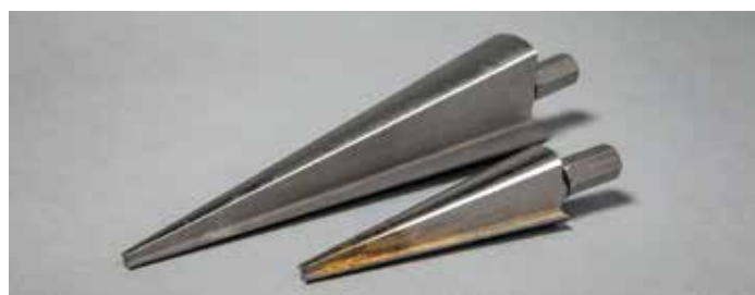
Tapered reamers don't match the angles perfectly but they get close enough to seat and support the pen
