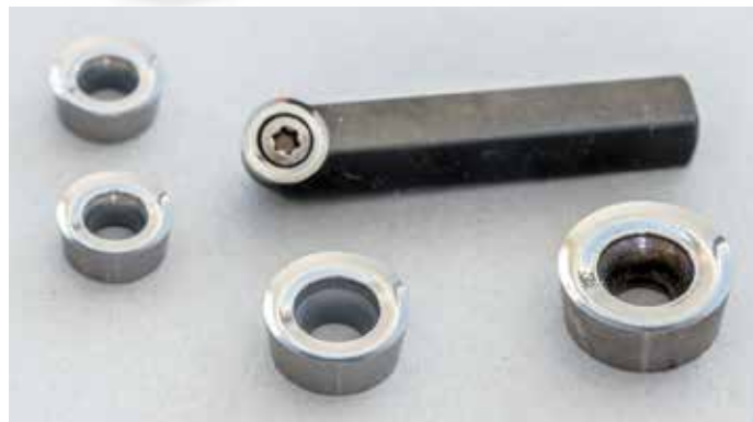
AZ Carbide's newest offering is a large carbide scraper that mounts to many systems, offering a host of contours to engage
