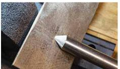
Regardless of the wheel media, the grit size is imparted on the steel of every tool it touches, creating the serrated cutting edge
