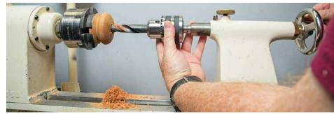
A Morse taper was never intended to provide high retraction force. Good practice requires the operator to provide this force
