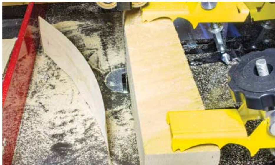
Once a re-sawing blade is installed and tracking, slicing veneer and steambending stock or trim is a breeze. It's nice to leave it set up and ready
