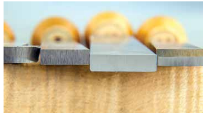
You can see the difference in the grit patterns imparted on the faces of these scrapers between the 60-grit and 200-grit wheels used to sharpen them
