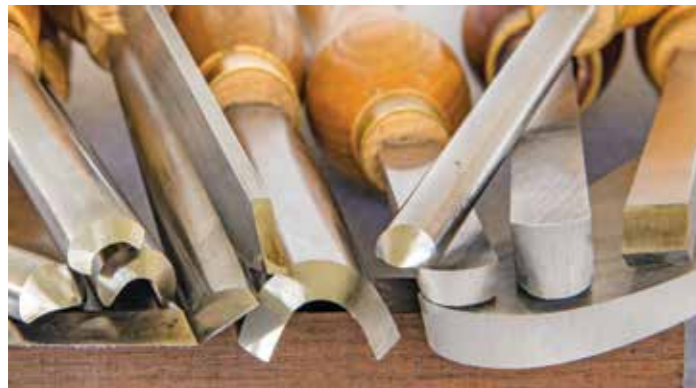
The grit of the wheel used for sharpening will be imparted to the tool edge as it is sharpened. For finer striations, use a finer-grit wheel
