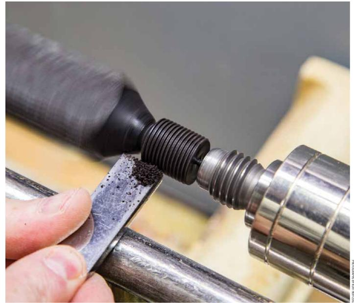
Hand chasing threads is an easy skill to master with a bit of practice. Like the skew, there are only a couple of rules
