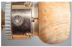
Good practice for chuck mounting is to mount flush on the tenon shoulder with a good tenon depth, without touching the bottom of the chuck
