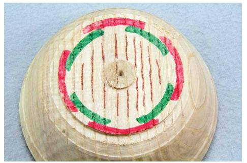
The best strength and durability for clamping on a tenon is with the chuck jaws angled to the grain (green) as opposed to on axis and across the grain (red)
