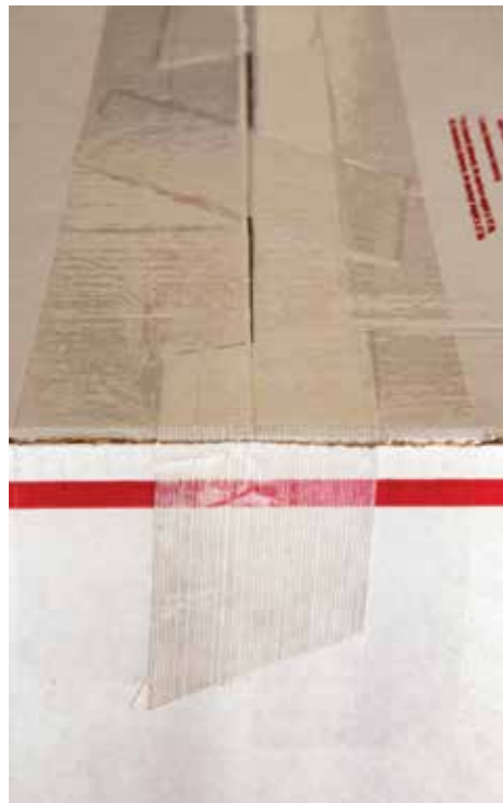
I use much higher-cost tape such as fibreglass reinforced in a few areas for needed strength, then use the traditional clear plastic strapping tape over top
