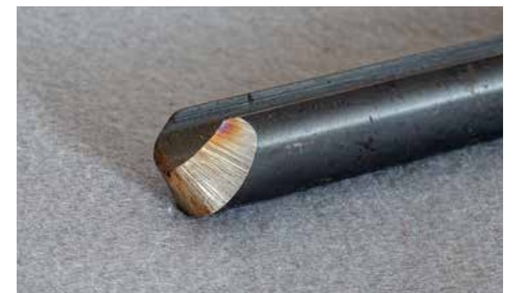
For HSS and beyond, if your tool is shaped correctly and cuts well, you can accept any unsightly heating discoloration as cosmetic only
