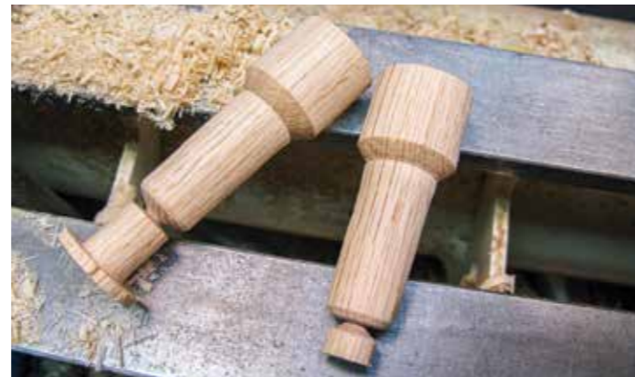
Lop off the scrap at the ends of the tapers on the bandsaw and these plugs will provide years of service
