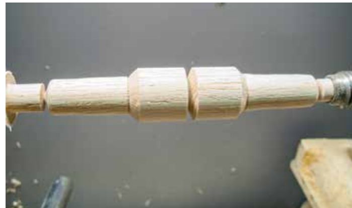
You can turn a couple of plugs simultaneously between centres using scrap wood. Here I'm making my tapers from a length of white oak
