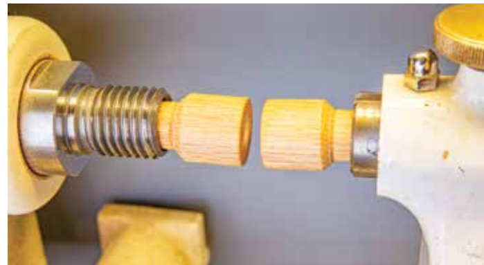
Since they will reference and perfect align on the tapered face on the shoulder, I make my plugs removable by hand with a very sloppy taper diameter fit
