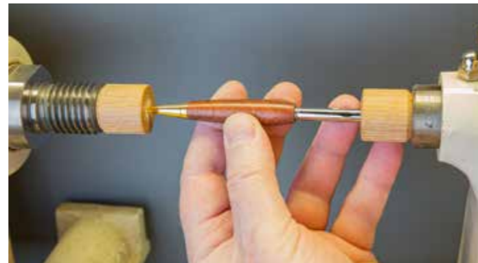
Your lathe is the greatest pen press you can ever have. It is already there and exhibits all the attributes of a press
