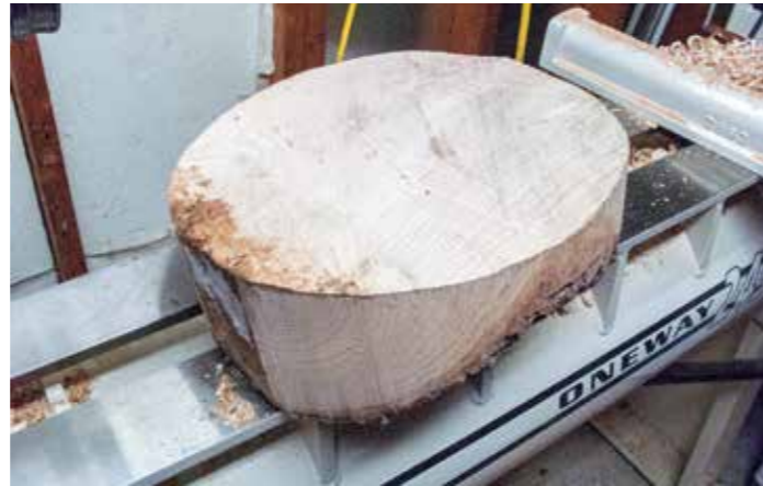
Unevenly weighted blanks such as this large, natural-edge bowl blank will benefit with plenty of horsepower used for low-rpm turning
