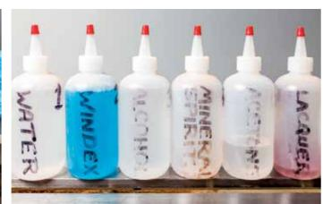
A simple example of my working containers for solvents used in the shop, numbered one to six, the weakest being water then through to my lacquer thinner. Each is in a marked polyethylene chemical bottle with tight-fit cap
