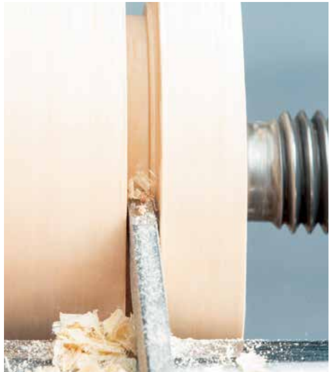
You can prevent side wall burning of a straight-walled parting tool by stair stepping your parting cuts, providing clearance width as you cut deeper
