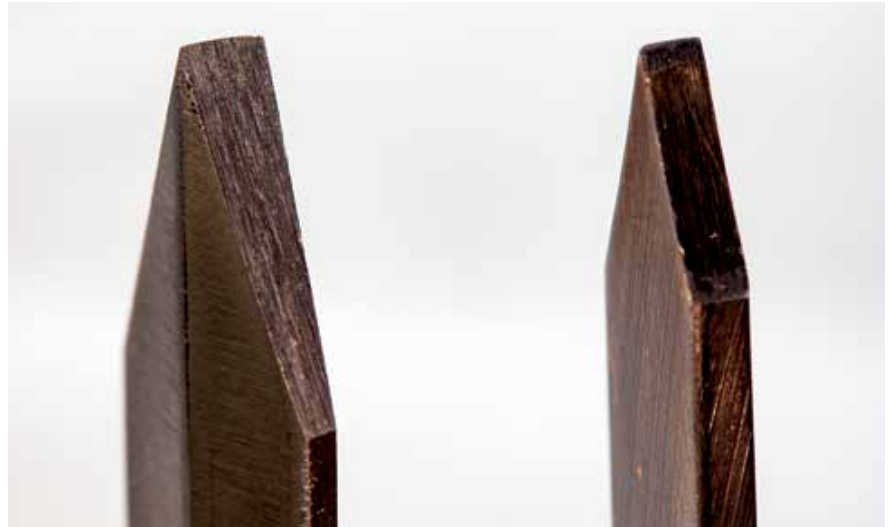
A diamond shape parting tool cuts its own clearance but does need to have the grind meet at the diamond feature on the shaft. Not needed on the standard tool
