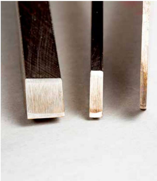
I favour straight-walled parting tools and my kit contains a 1.5mm, a 3mm, and a 10mm beading/parting tool for larger work
