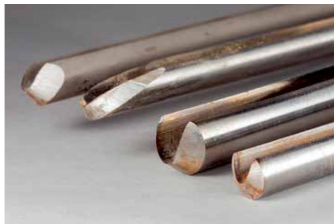
My bowl gouge kit contains (L to R) a fingernail grind bowl gouge, an Ellsworth gouge, a standard grind bowl gouge, and a bottom cutting bowl gouge
