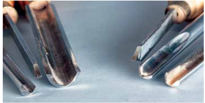
Left: Starting spindle turning kit of spindle gouge, parting tool, and roughing spindle gouge. Right: Starting bowl kit of a parting tool, spindle gouge, and bowl gouge
