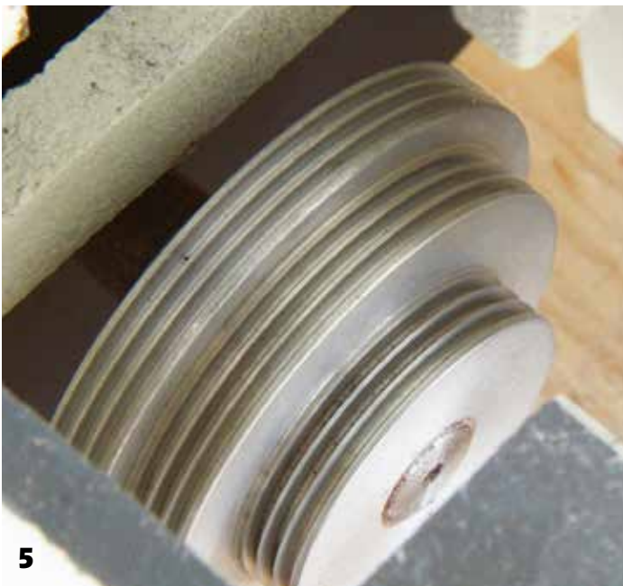
4 Properly aligned and tensioned, Poly-V belts provide excellent service and life. Here, the original belt, still serviceable with 20 years of use 5 One of the advantages of Poly-V belts is their ability to work well on much smaller pulleys than the traditional V belts 6 Quiet and requiring no real maintenance or adjustment after initial setting, proper-sized belts can easily transfer multiple horsepower to the spindle
