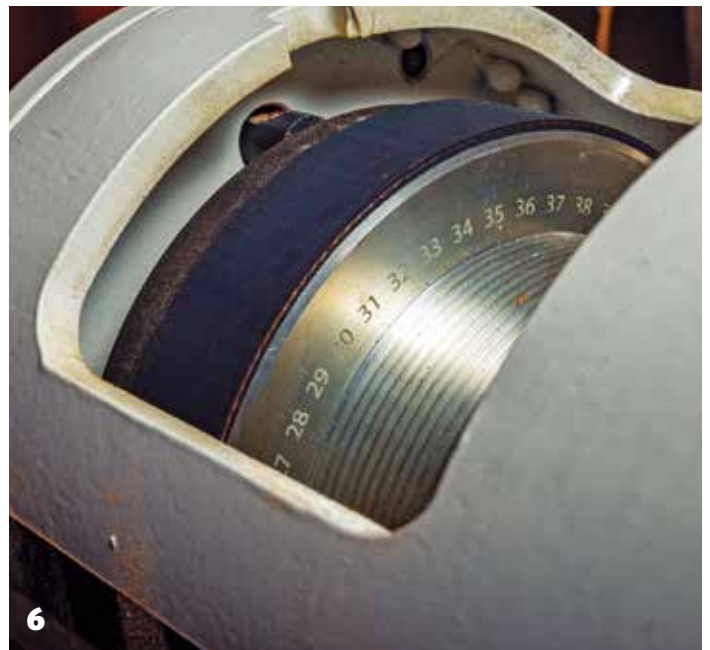
4 Properly aligned and tensioned, Poly-V belts provide excellent service and life. Here, the original belt, still serviceable with 20 years of use 5 One of the advantages of Poly-V belts is their ability to work well on much smaller pulleys than the traditional V belts 6 Quiet and requiring no real maintenance or adjustment after initial setting, proper-sized belts can easily transfer multiple horsepower to the spindle
