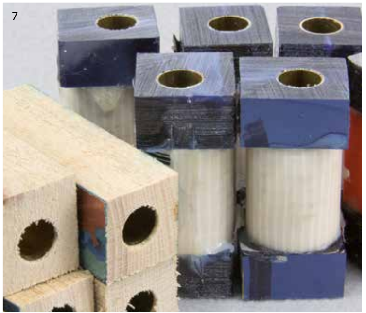
7 The gaps between the tube and the inner diameter can range from a very slight press to a slip fit, depending on the adhesive being used
