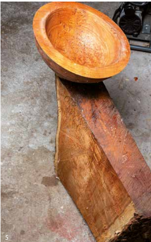
3 A piece of ambrosia maple I used to make a funeral urn. Turned and hollowed wet, allowed to dry, re-turned to true things up. Great result 4 A piece of Norfolk Island pine, debarked for no pest transport, waxed for storage until time for turning. Without sealing, it would self-destruct quickly 5 Anchorseal or equivalent works well for raw wood or in-process turnings. First turned, sealed, allowed to dry slowly, and then re-turned to finish
