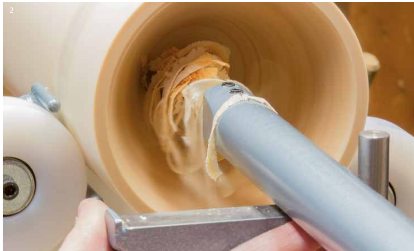
1 One of the advantages of green wood is the ability to get blanks in larger sizes. Large, dry blocks of wood are difficult – read 'expensive' – to obtain 2 Whether freehand turning or using a hollowing bar, green wood is a joy to turn. Usually cuts like soap with long curls that spray sap all over the place
