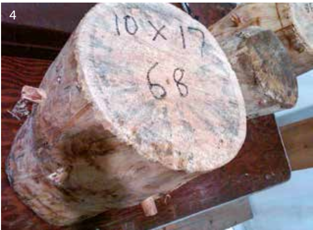
3 A piece of ambrosia maple I used to make a funeral urn. Turned and hollowed wet, allowed to dry, re-turned to true things up. Great result 4 A piece of Norfolk Island pine, debarked for no pest transport, waxed for storage until time for turning. Without sealing, it would self-destruct quickly 5 Anchorseal or equivalent works well for raw wood or in-process turnings. First turned, sealed, allowed to dry slowly, and then re-turned to finish
