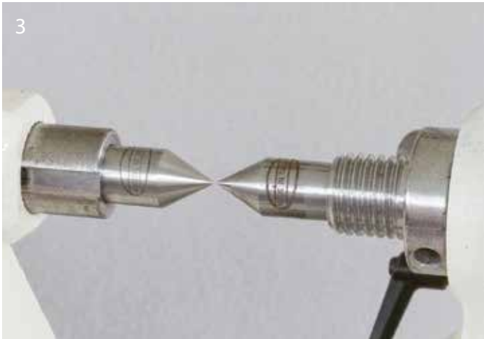
3 Use a dead centre in the head and tailstock. Slide them together carefully until they almost touch
