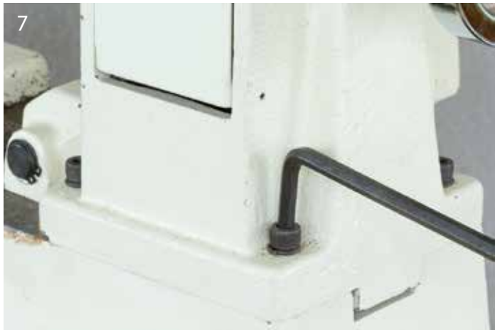
7 Loosen the headstock screws and orient side to side, front to back, or axis shift. Up and down can be shimmed as needed. Open holes or file if required
