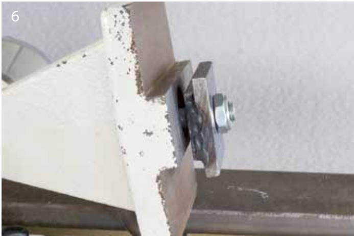
6 There is no easy alignment adjustment capability on the tailcentre. Because the alignment varies somewhat with each lock up, you get whatever it is
