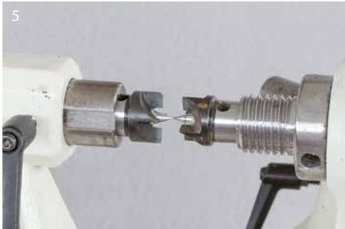
5 You can also use spur centres provided the points are sharp and not damaged or bent. They work, but I favour the dead centres for the few bucks cost
