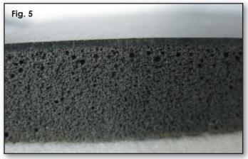
A cross section of the Ground Floor Packaging mat showing the hard top skin, which is bonded with the foam below.
