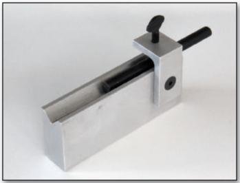
The sanding block is designed to clamp the proper punch or dowel, allowing for the ID guidance of the pen blank being perpendicularly sanded to the glued-in brass.
