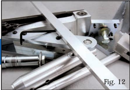
The Gizmo is made from quality parts and the design lends itself to different-size lathes with only one simple part change—the mounting bracket.
