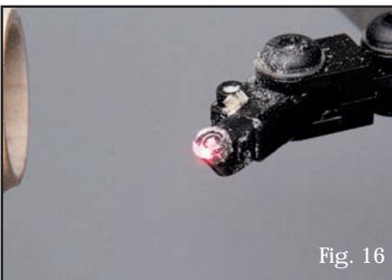
There is a flexible laser system to indicate the cutter position or wall thickness in accordance with your wishes.
