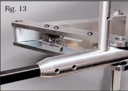
The Gizmo has a unique construction in the articulated arm segment. It is a fabrication that works in principle similar to an “I” beam.
