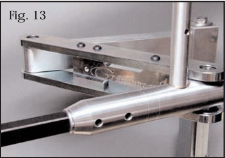
Fig. 13 The Gizmo has a unique construction in the articulated arm segment. It is a fabrication that works in principle similar to an “I” beam.
