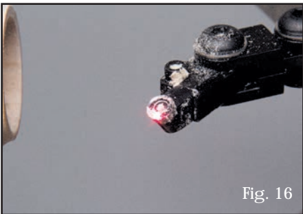
Fig. 16 There is a flexible laser system to indicate the cutter position or wall thickness in accordance with your wishes.
