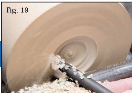
The #1 Mini Hercules square tool shaft helps keep the tool flat on the rest during use. Both Osprey tools cut nicely when rotated to present a skewed cutting edge for an extremely clean as cut surface finish.
