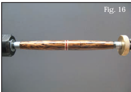
Fig. 16 The better the preparation of the blank to accept a finish, the better the finish will turn out because any flaw of any kind will be highlighted under the finish.
