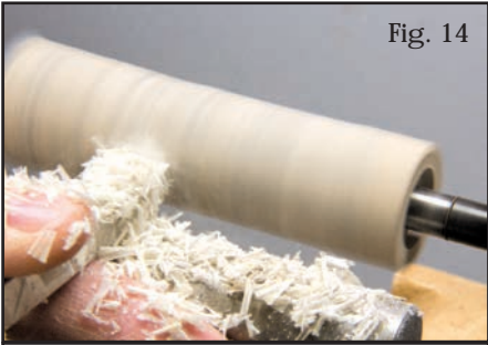
Fig. 14 For those who would prefer to purchase their sharp edge rather than grind it, any of the carbide cutter tools can be used to turn pens.
