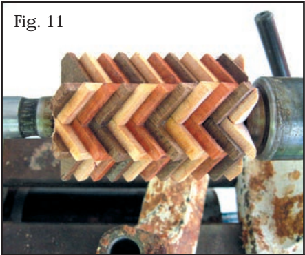
Fig. 11 The methodology of cutting and gluing up segmented work can take many forms. This blank in progress is by Joe Schneider.
