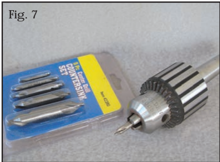
Fig. 7 A center drill, basically a rigid short drill point, is a modest-priced method for creating a drill starting point on a lathe. Sets are available at discount auto and machinery suppliers.
