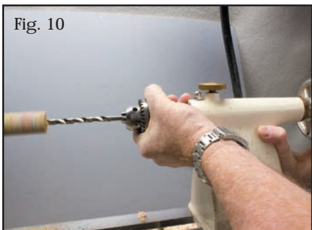
Fig. 10 When drilling with the tailstock unfastened, the drill will find the path of least resistance as it drills. Speeds and feeds along with breaking the chip still apply. It is key to hold the drill chuck for safety throughout the process.
