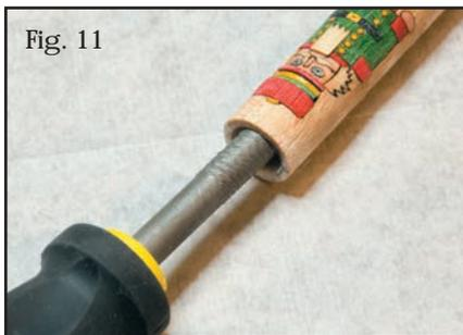
When the assembly is complete, the tube is pushed out and the inside of the wooden blank is cleaned up with a rat-tail file.
