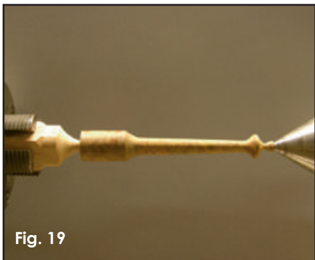
Fig. 19 Bring up the tailstock for additional support.
