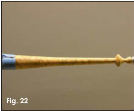
Blue tape aids in securing the blank to the headstock mandrel.
