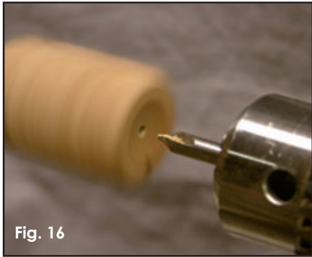
Fig. 16 A center drill works best to locate the new center on this end of the blank.
