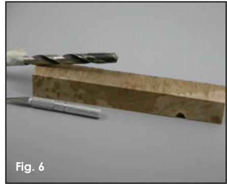
Fig. 6 A little tape on the bit acts as a depth gauge.
