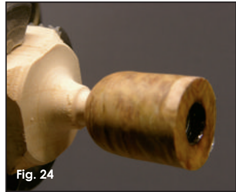
Retract the tailstock once rough shaping is completed.
