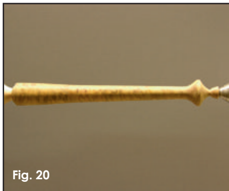
Fig. 20 Turn the other end to approximate shape.
