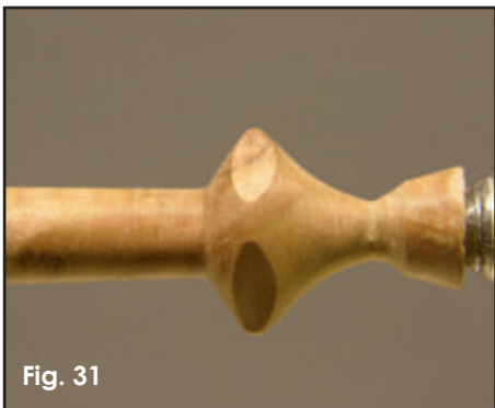
Flats prevent the knife from rolling around.
