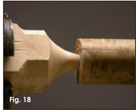
Fig. 18 Make a jam chuck from a scrap piece of stock.
