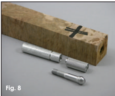
Fig. 8 Make witness marks to help with future alignment.
